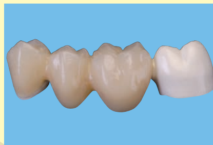
The polishing properties of the veneer composite and of the BioHPP as fully-anatomical chewing surfaces are so good that a rough depth in BioHPP of only 0.018 \mu\text{m} R_A can be achieved.
