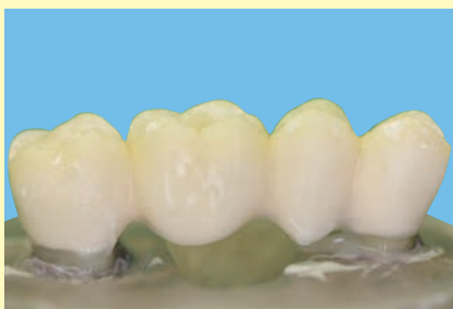
4-part bridge made from BioHPP veneered with visio.lign with mobile socket with vario-link II prior to the chewing simulation test.
